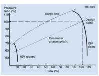
inlet guide vanes of both compressor stages, still maintaining the high efficiency of the unit.
